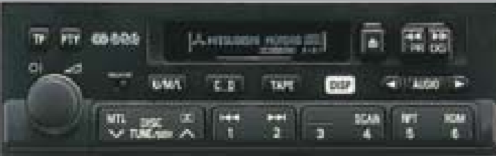
PH-2000 Radio/cassette player with RDS-EON tuner, CD changer control buttons, trip computer mode switch, telephone mute preparation and detachable front key-panel, 4 x 30W. MZ312719
