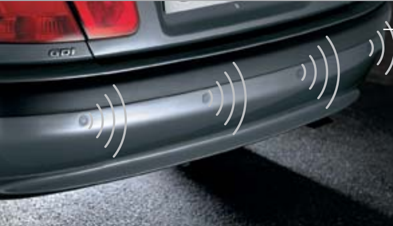
Rear parking assistance Supports driving backwards with audible distance indication. Sensors can be painted in body colour. MZ312947
